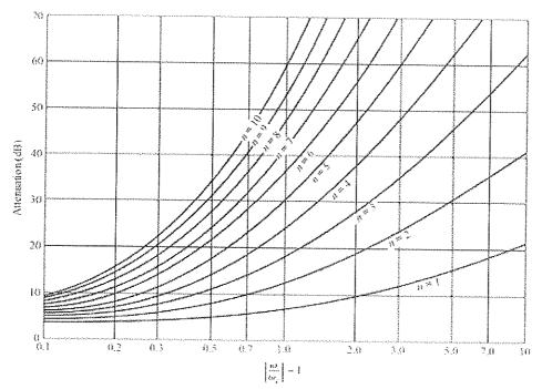
Attenuation versus normalized frequency for maximally flat filter prototypes. Adapted from G. L. Matthaei, L. Young, and E. M. T. Jones, Microwice Filters, Impedance-Matching Networks, and Coupling Structures, Artech House, Dedhum, Mass., 1980, with permission.
